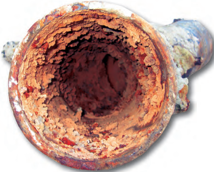
Looking down a Toronto city water main, removed in July, 2007
